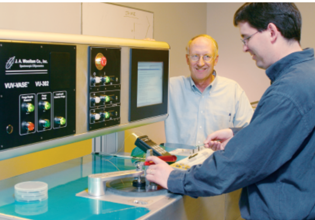
Woollam watches while James Hilfiker loads a sample into a spectroscopic ellipsometer that covers the vacuum ultraviolet to the near infrared.
