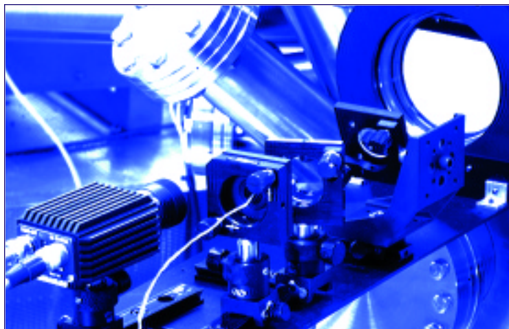
Figure 1. Multibeam optical sensor mounted on a commercial thin-film deposition system.
