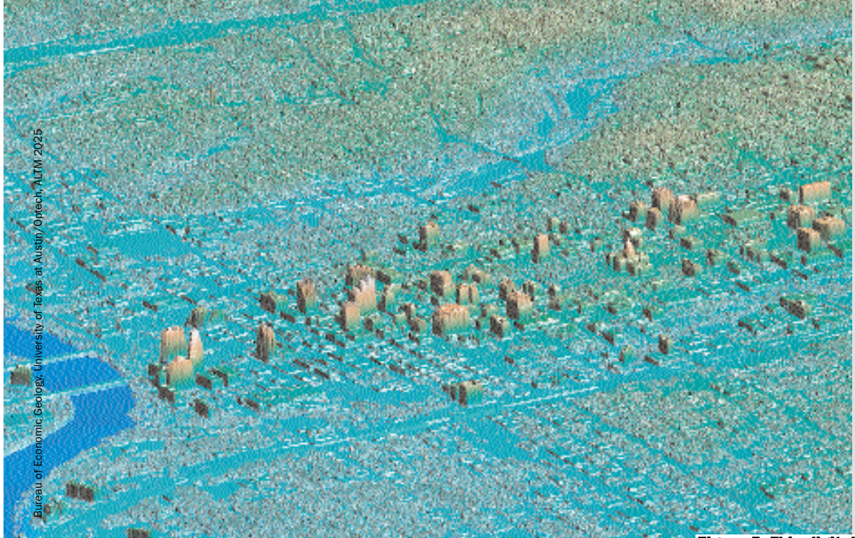
Figure 5. This digital elevation model of Austin, Texas, was computed to a resolution of 1 m \times 1 m from more than 180 million elevation points.
