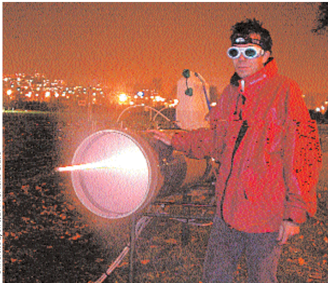
On a foggy night outside Lyon, France, when regular laser beams would be scattered, stable filaments of 400-mJ, 100-fs laser pulses are detected by a cloud chamber over a distance of 50 m.
