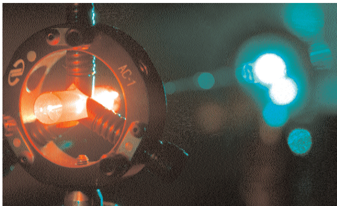
Light has been observed to travel at only 91 m/s in a crystal of alexandrite at room temperature in an experiment at the Institute of Optics, which has also slowed light in this ruby crystal.
